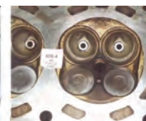
Combustion chamber after P.i. treatment.
