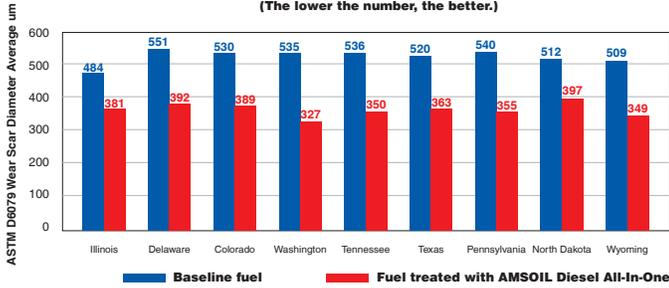
The ASTM D975 diesel fuel standard specifies a wear scar below 520 µm in ASTM D6079 testing, while the Engine Manufacturers Association (EMA) specifies a wear scar below 460 µm. Testing reveals AMSOIL Diesel All-In-One provides significant lubricity improvement in diesel fuels found across the U.S., delivering improved wear protection.
